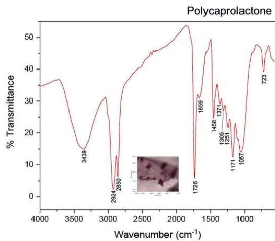
Figure S2. Infrared spectra of samples of poly(vinyl chloride), polymethyl methacrylate, polystyrene, polyurethane and polycaprolactone.
