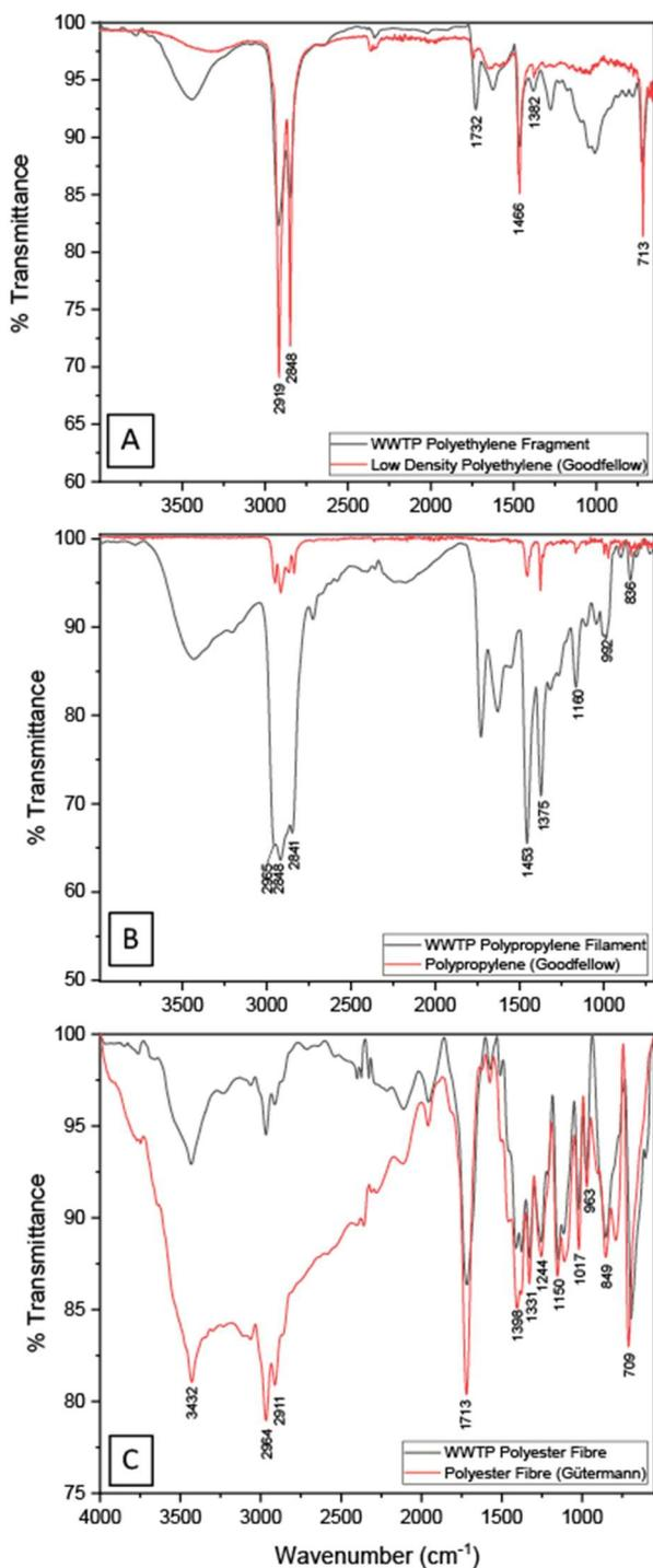
**Figure 3.** Infrared spectra of environmental samples and their corresponding reference standards for polyethylene (A), polypropylene (B), and a polyester fibre (C).
